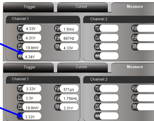
Figure 2-31 P14 High Signal Voltage Measurement with LED Circuit Load
