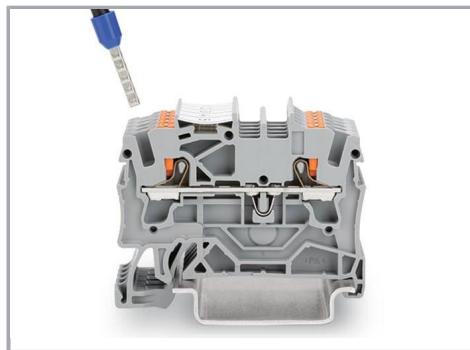
Push-in termination of solid and ferruled conductors
