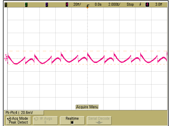
Figure 2: ADO300-48S05 Output Ripple and Noise Measurement see figure 13 for test configuration Ch 3: Vo (2uS/div, 20mV/div)
