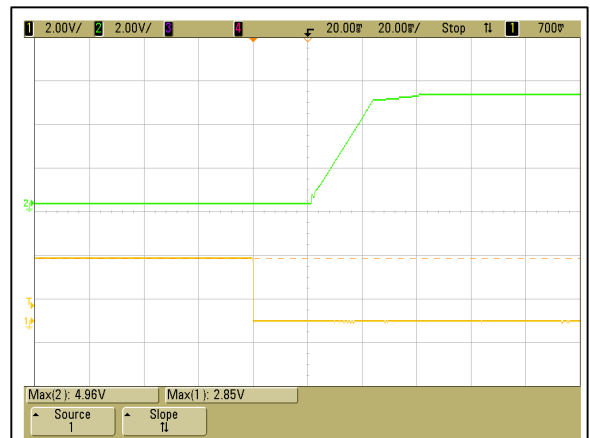
Figure 6: ADO300-48S05 Remote ON Waveform (5mS/div) see figure 12 for test configuration Ch 2: Vo (2V/div) Ch 1: Remote OFF (2V/div)
