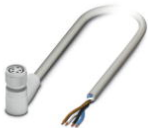
Sensor/actuator cable, 4-position, PP-EPDM halogen-free, gray RAL 7035, free cable end, on Socket angled M8, with 2 LEDs, cable length: 1.5 m, Hygienic design, with plastic knurl
