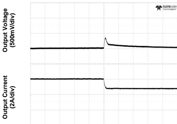
Figure 5. Transient Load Response (typical Vin, load current steps from 50% to 25% at a slew rate 0.1A/µs)
