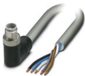
Power cable, 5-position, PVC, gray RAL 7001, Plug angled M12, L-coded, on free cable end, cable length: 1.5 m, for direct current up to 16 A/63 V
