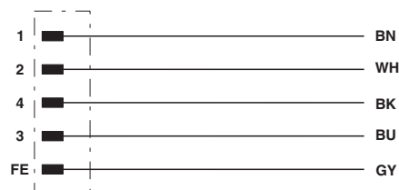
Contact assignment of the M12 plug
