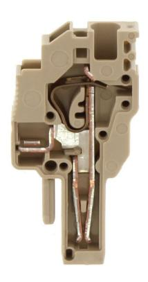
Feed-through terminal, Tension-spring connection, Mounting type: Plug in, Rated cross-section: 2.5 mm², Width: 5.1 mm, Colour: Beige
