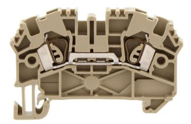
Ex feed-through terminal ATEX-certified, Tension-spring connection, Mounting type: Mounting rail TS 35/7.5, Rated cross-section: 2.5 mm<sup>2</sup>, Width: 5.1 mm, Colour: Beige
