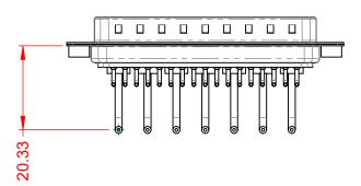
POWER/CO-AX CONTACT RATING:10A (CURRENT)(IF PRESENT)SIGNAL CONTACT CURRENT RATING:5A PER CONTACTSIGNAL CONTACT RESISTANCE: $10m\Omega$  MAX.INSULATOR RESISTANCE:5000MΩ min.DIELECTRICDIELECTRIC
