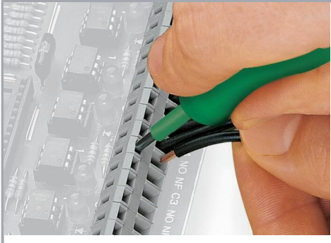
Inserting a conductor via 3.5 mm screwdriver.
