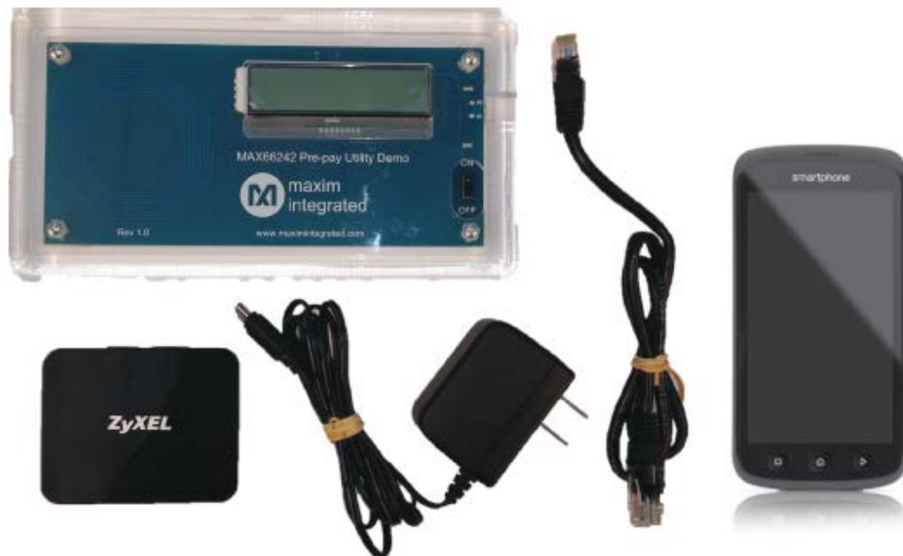
Figure 3. The prepay utility demonstration platform presented here features the MAX66242 secure authenticator tag and a MAXQ610 microcontroller (not seen here).
