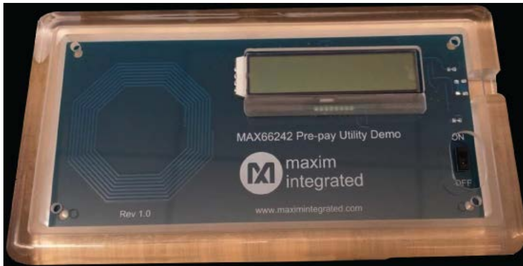
Figure 2. Demo board for a NFC-based prepay home display unit (HDU). The HDU communicates with the utility's back office to update the remaining energy credits. The transaction uses powerline communication (PLC) across the home's existing electric wiring.
