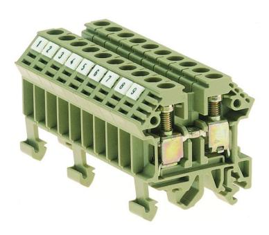
Feed-through terminal/block variant, Screw connection, Mounting type:Mounting rail TS 35/7.5 and TS 32, Rated cross-section: 10 mm², Colour: Beige
