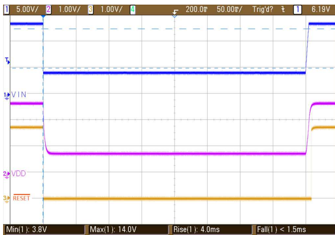
Figure 51. TPS3840-Q1 Warm-Start Test Pulse
