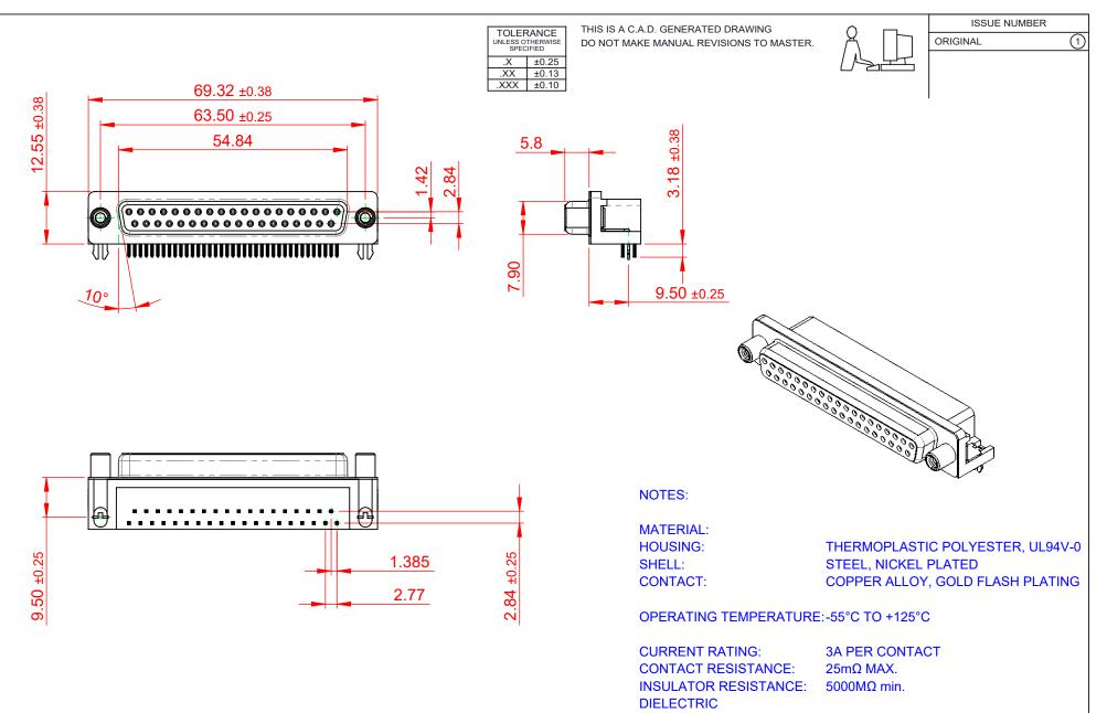
WITHSTANDING VOLTAGE: 1000V AC rms
