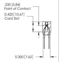
725 Series Ultra-Mate Card Edge Connector - Press Fit Part Number: 725-050-540-201
