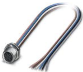
Sensor/actuator flush-type socket, 6-pos., M8, rear/screw mounting with M10 fastening thread, with 0.5 m TPE litz wire, 6 x 0.14 mm 2
