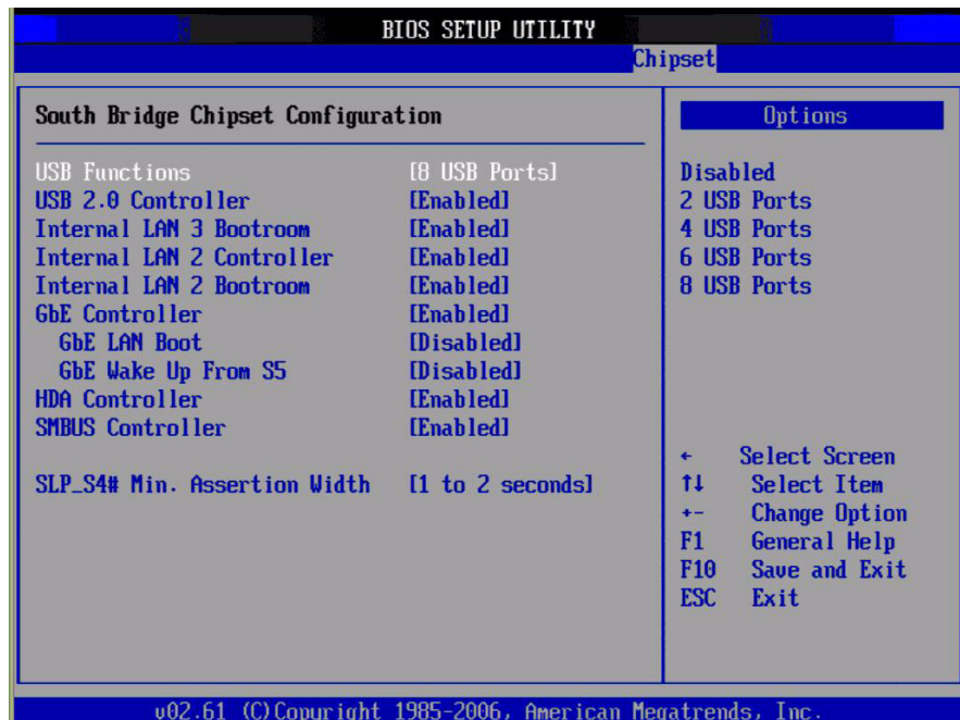
Figure 3.27 South Bridge Configuration
