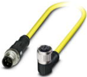
Sensor/actuator cable, 4-position, PVC, yellow, Plug straight M12 SPEEDCON, A-coded, on Socket angled M12 SPEEDCON, A-coded, cable length: 1.5 m
