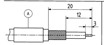
Slide ferrule A onto cable. Prepare cable according to diagram. CAUTION: Do not damage braid, dielectric and inner conductor of cable!
