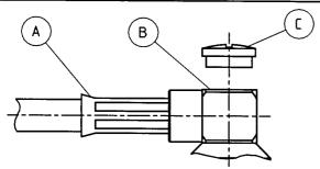
Slide ferrule A over braid and crimp as close to connector body B as possible.
