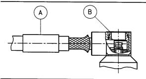
Splay out braid and insert cable in connector body B. CAUTION: Ensure that braid lies above the crimp neck.
