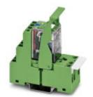
Preassembled relay modules with screw connection, consisting of: relay base, industrial relay with integrated LED and engage/disengage manual actuate lever, varistor protective module, and retaining bracket. Input voltage: 24 V AC, two PDTs, 10 A
