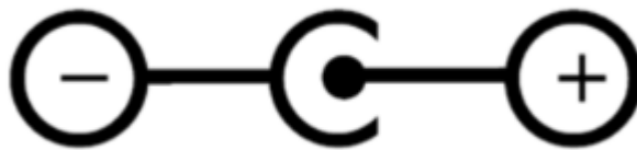
Figure 4 • Power Supply Cable Polarity
