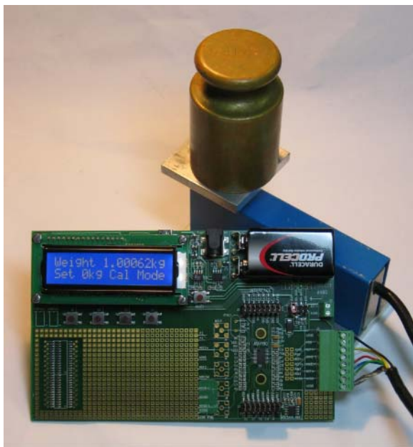
Figure 2. Weigh Scale System Using the AD7192
