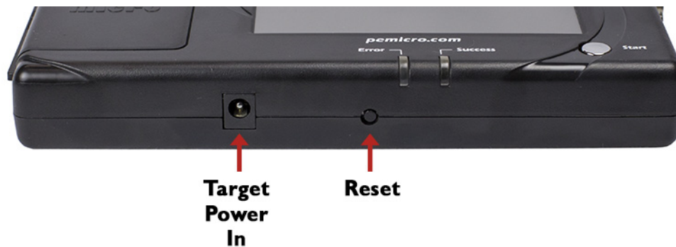
Figure 3-3: CYCLONE FX Front Side View
