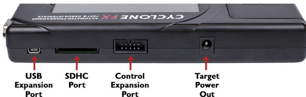
Figure 3-4: CYCLONE FX Rear Side View
