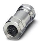
Connector, 5-position, shielded, Socket straight M12, A-coded, Screw connection, knurl material: Stainless steel 1.4404, cable gland M16, external cable diameter 5.5 mm ... 8.6 mm
