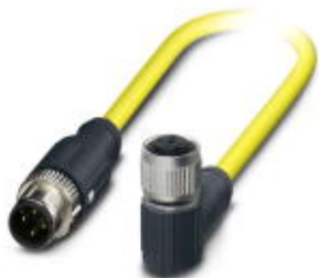
Sensor/actuator cable, 4-position, PVC, yellow, shielded, Plug straight M12 SPEEDCON, A-coded, on Socket angled M12 SPEEDCON, A-coded, cable length: 1.5 m
