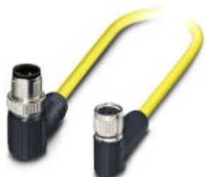
Sensor/actuator cable, 4-position, PVC, yellow, shielded, Plug angled M12 SPEEDCON, A-coded, on Socket angled M8, cable length: 0.5 m
