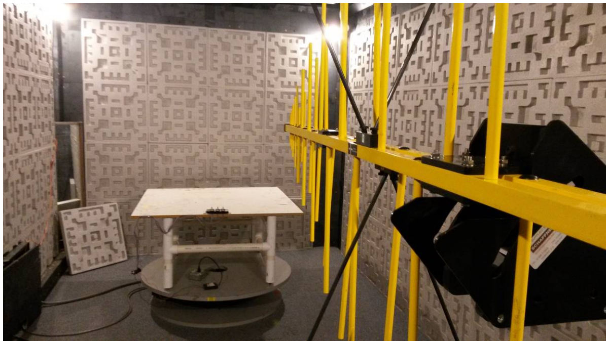
Figure 11 – Radiated Emissions Test Setup
