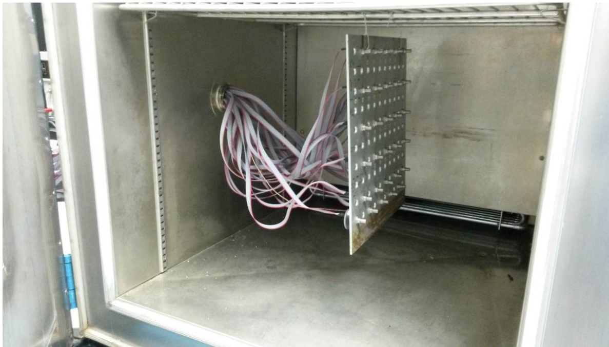
Figure 1 – Four Corners Test Setup (DUTs in chamber)
