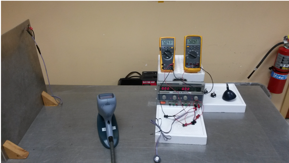
Figure 29 – Electrostatic Discharge Test Setup
