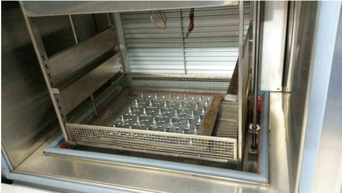
Figure 4 – Thermal Shock Test Setup (DUTs in chamber)
