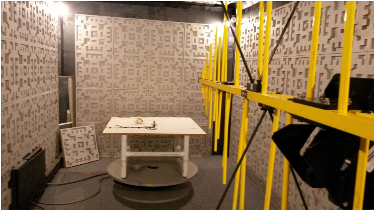
Figure 20 – Radiated Immunity Test Setup
