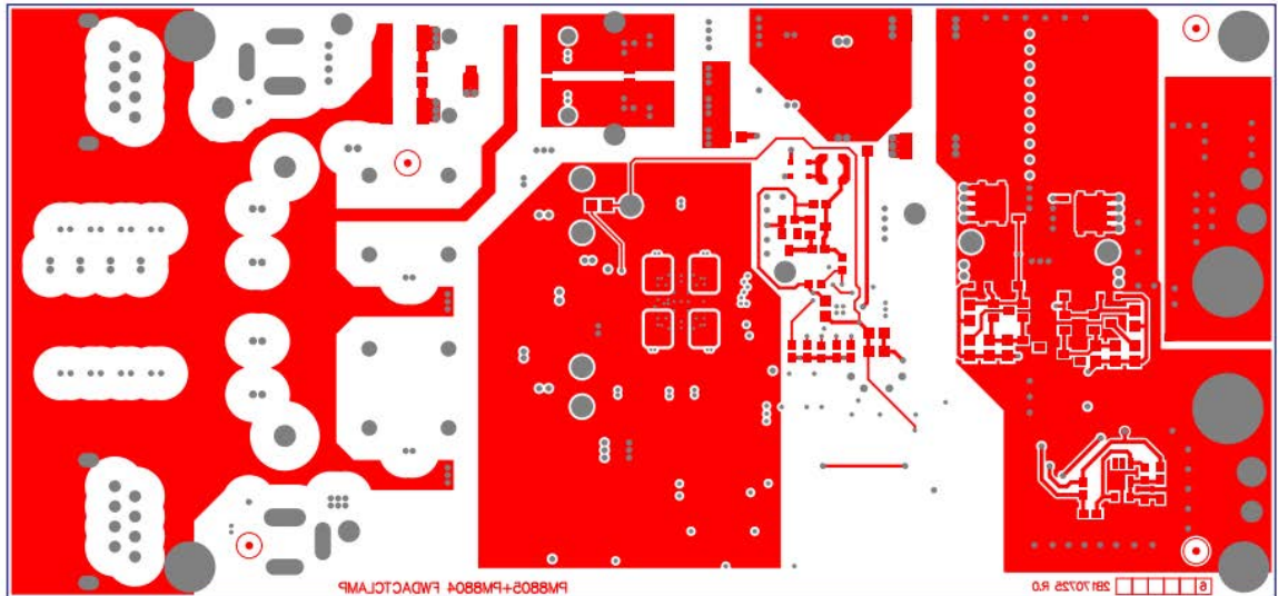
Figure 37. STEVAL-POE003V1 reference design: PCB layer 6
