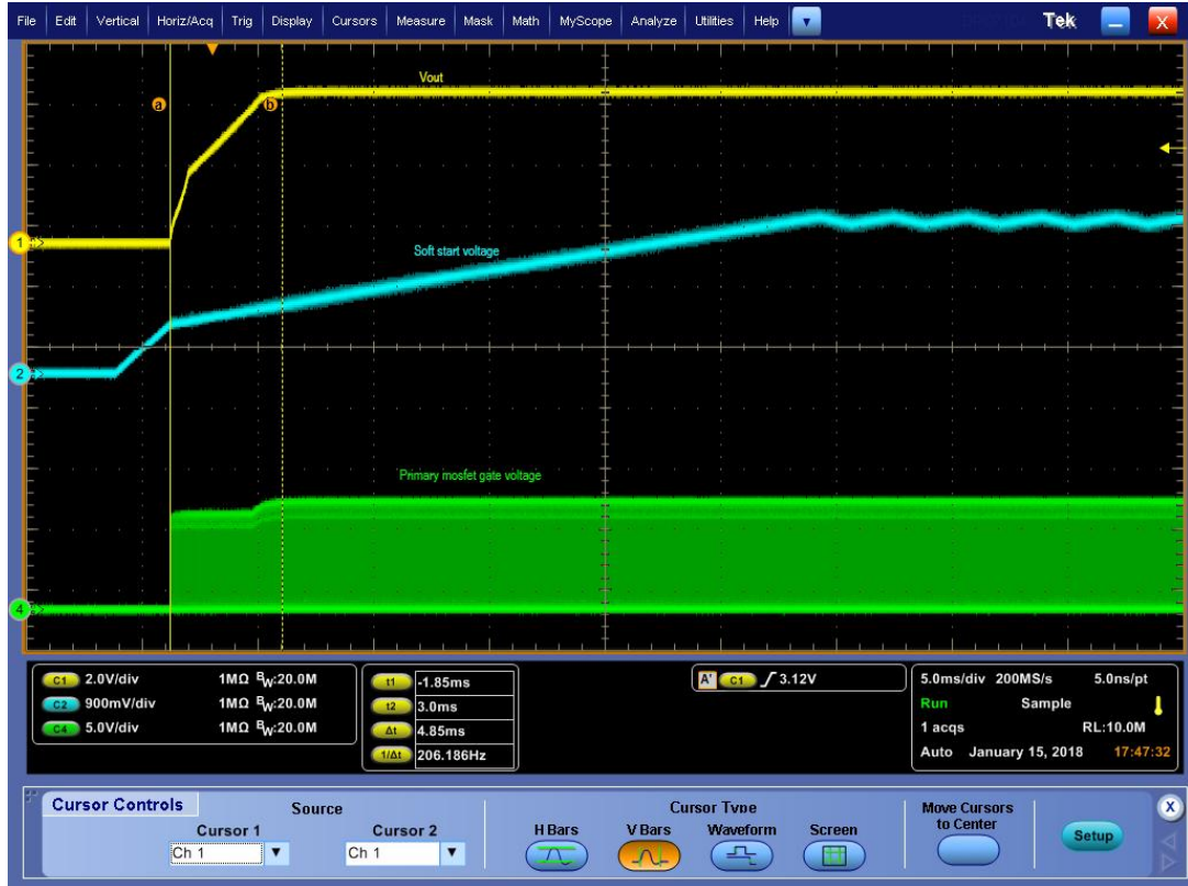
Figure 11. Output voltage at startup: I out at no load, V in = 48 V
