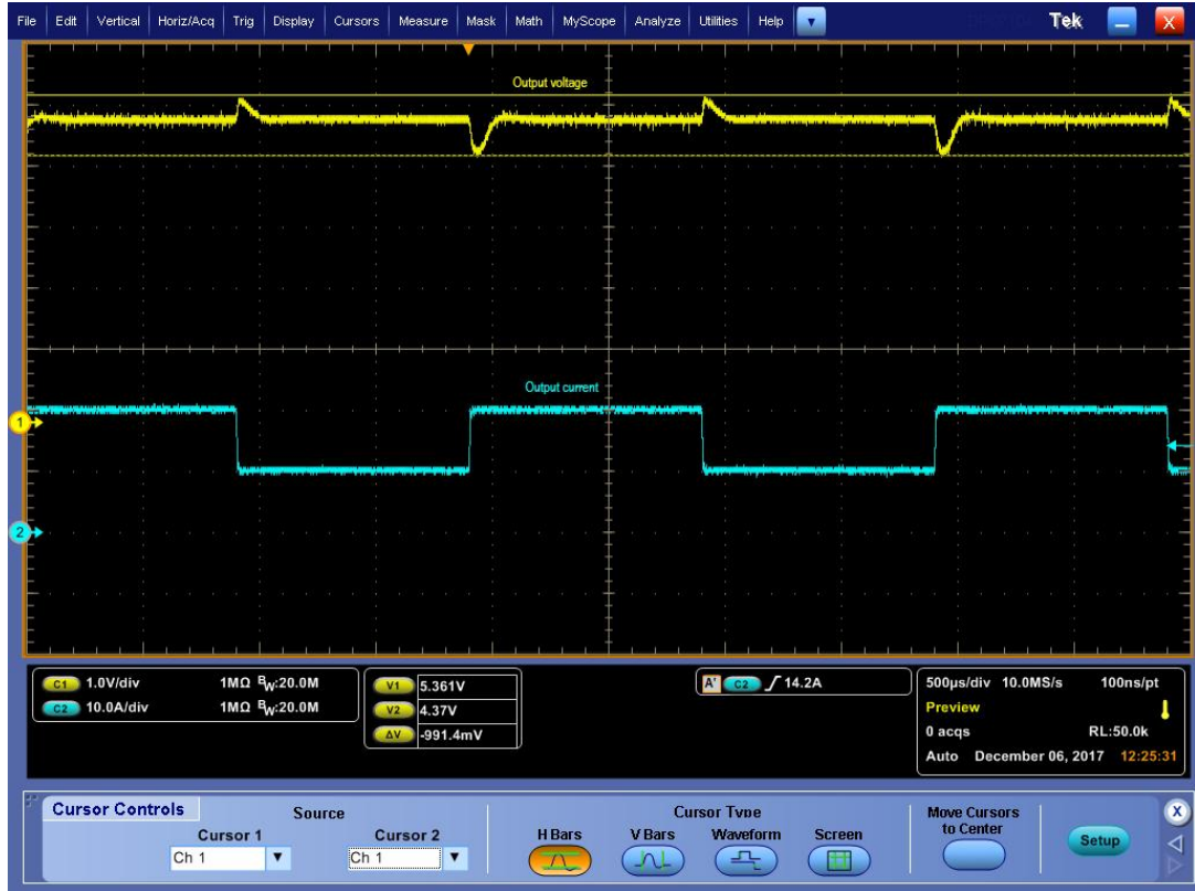
Figure 20. Load transient: I out =10 to 20 A, V in = 48 V
