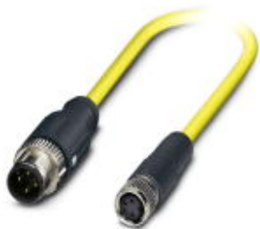
Sensor/actuator cable, 4-position, PVC, yellow, shielded, Plug straight M12 SPEEDCON, A-coded, on Socket straight M8, cable length: 0.5 m
