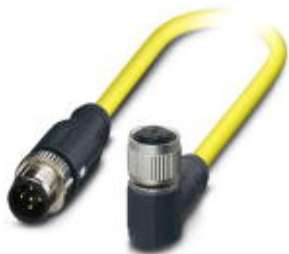
Sensor/actuator cable, 5-position, PVC, yellow, shielded, Plug straight M12 SPEEDCON, A-coded, on Socket angled M12 SPEEDCON, A-coded, cable length: 1.5 m
