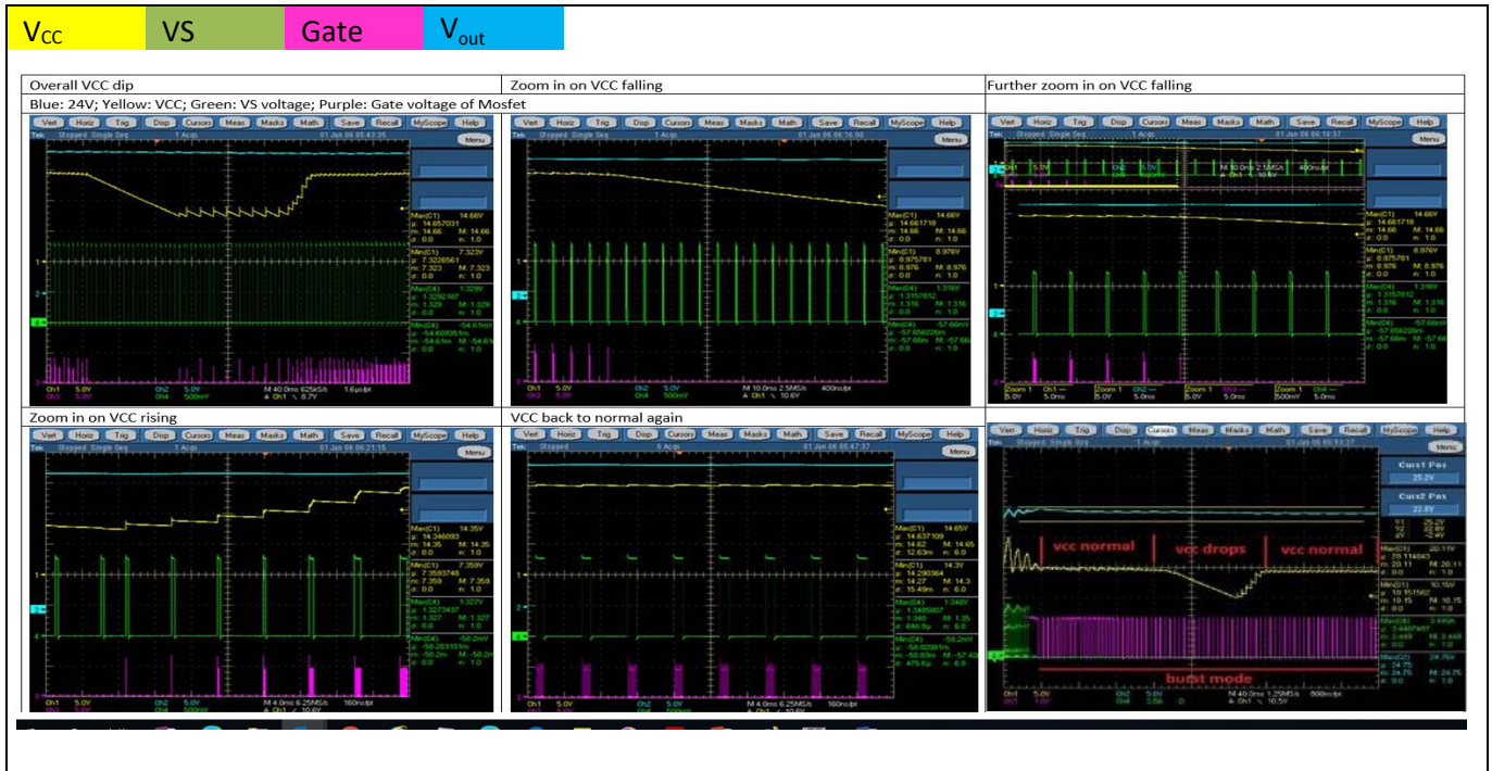
Figure 38 V_{CC} maintainance mode if V_{CC} drops too low, with minimum impact on output; V_S signal shows wake-ups and gate-only pulses if necessary
