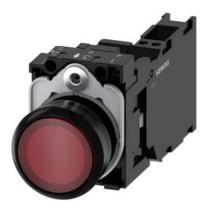
Illuminated pushbutton, 22 mm, round, plastic, red, pushbutton, flat, momentary contact type, with holder, 1 NO+1 NC, LED module with integrated LED 24 V AC/DC, spring-type terminal, with laser labeling, symbol number according to, ISO 7000 or IEC 60417
