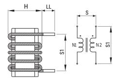
General InformationSeriesSC-DStyleThrough-HoleRoHSYesNotesLead Spacing (S/S1) Are For Reference Only.MiscellaneousTemperature Rise Maximum: 40 K.CoreNi-Zn Ferrite
