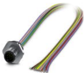
Flush-type connector, Universal, 17-position, Plug, M12, A-coded, Front mounting, M16 x 1.5, Individual wires, cable length: 0.5 m
