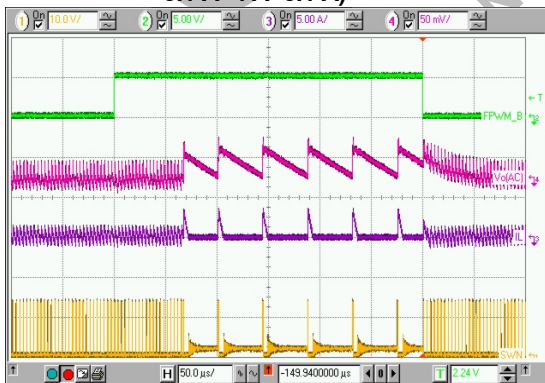
Top: FPWM#, FPWM# Signal, (5V/div) Middle 1: Vo1, CH1 Output Voltage Ripple, (50mV/div) Middle 2: iL1, CH1 Inductor Current, (5A/div) Bottom: SWN1, CH1 Switching Node Voltage, (10V/div) Time: 50µs/div
