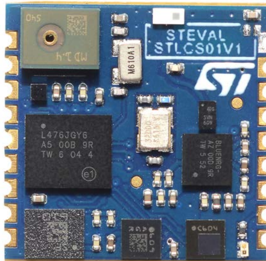
Figure 10. STEVAL-STLCS01V1 SensorTile module
