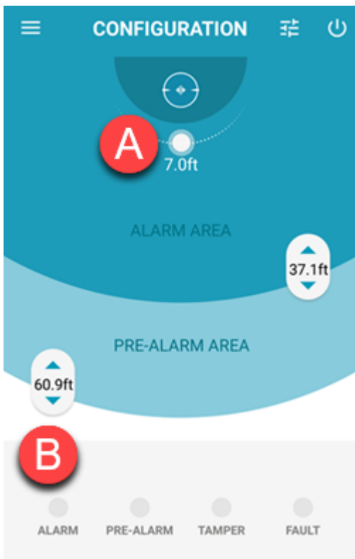
Wrong calibration. Calibration value too high.
