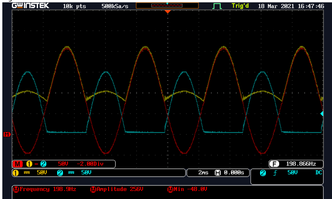
Figure 24 oscilloscope screenshot while probing a Highdriver at 250Vpp & 200Hz with load (mp6) attached
