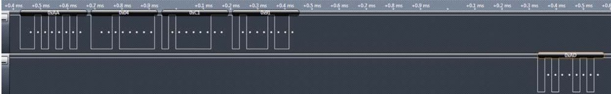
Figure 2. SSI select target logic waveform.
