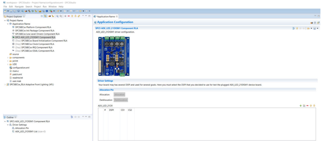
Figure 60. Add LED driver component to project
