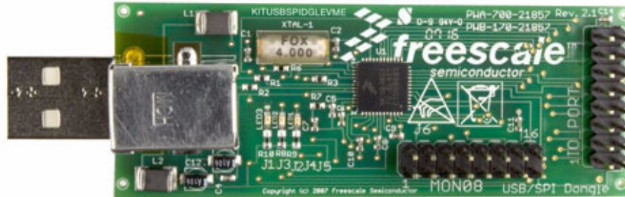
Figure 6. KITUSBSPIDGLEVME Interface Dongle
