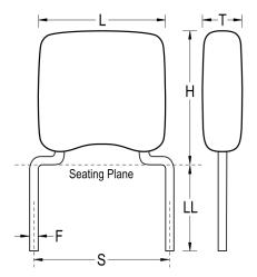
**General Information** Series GoldMax 300 Comm X8L HT150C Style Radial Description "GoldMax, Commercial Standard" RoHS Yes Termination Tin Failure Rate N/A AEC-Q200 No Halogen Free Yes
