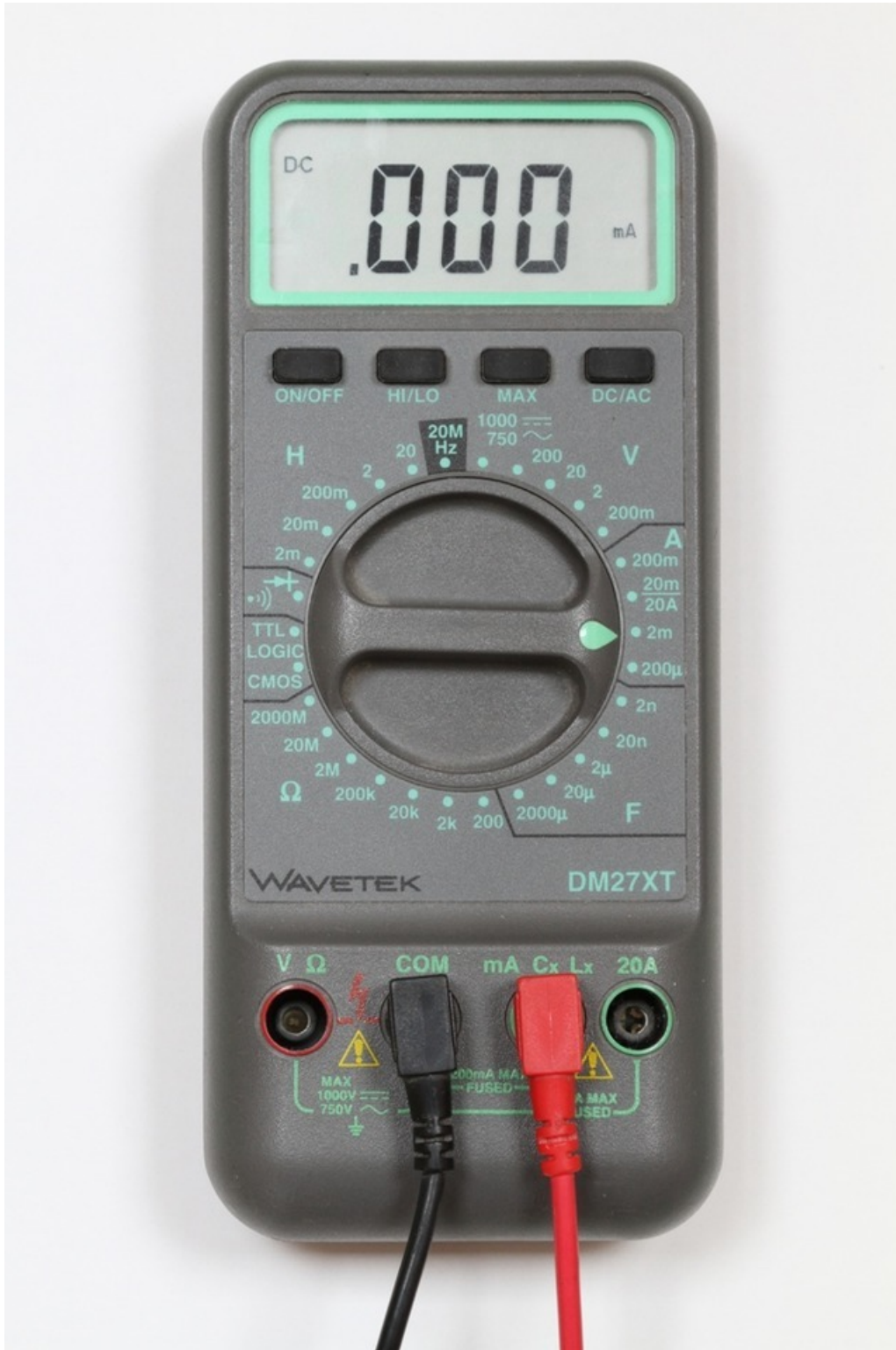
Here we are using the 0-200mA jack to make a measurement in the 2mA range.
