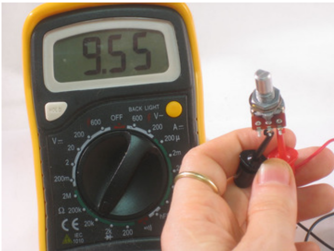
Maximum value is 9.5KΩ (it should be around 10KΩ)
