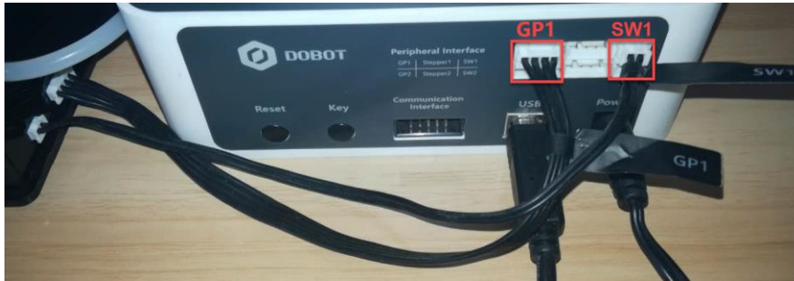
Figure 1.7 connect the air pump to Dobot Magician
