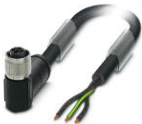
Power cable, 3-position, PVC, black, free cable end, on Socket angled M12, S-coded, cable length: 10 m, for AC current up to 16 A/230 V
