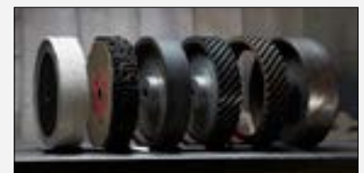
Figure 6 | Image illustrating the range of materials and configurations of contact wheels.
