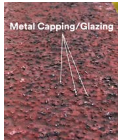
Figure 4 | Image depicts an example of glazing which can result from not applying enough pressure.
