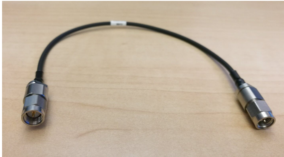
Figure 34: SMA to SMA Cable: Carlisle TM40-0159-00 6"
