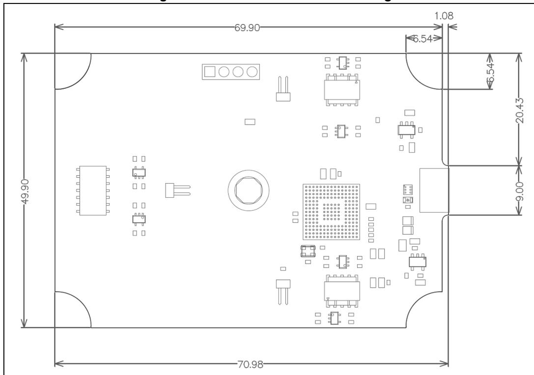
Figure 12. MB1440 mechanical drawing
