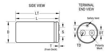
General Information Series ALS30 Dielectric Aluminum Electrolytic Description Screw Terminal, Aluminum Electrolytic RoHS AEC-Q200 No Component 960 g Weight Dimensions D And L Include Sleeving. MS (MxH) = Notes M12x16. Mounting Clamp (Sold Separately): V11 Shelf Life 156 Weeks
